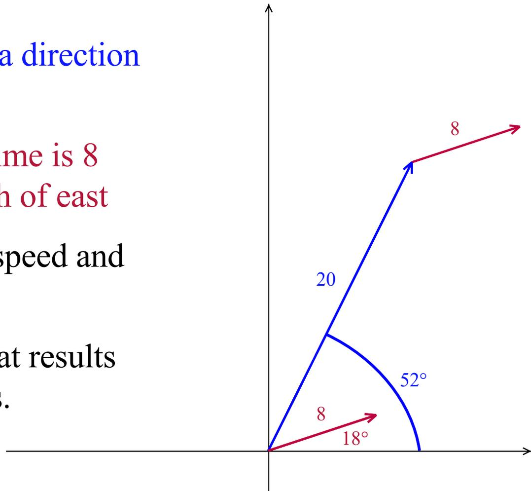
A boat is sailing at 20 mph with a direction of  $52^\circ$  north of east.
