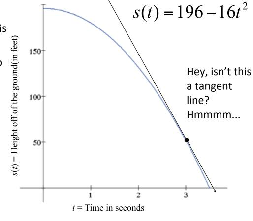
$$v = \lim_{t \to 3} \frac{196 - 16t^2 - (196 - 16 * 3^2)}{t - 3 \text{ sec}} \frac{\text{feet}}{\text{ }}$$
