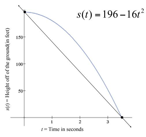
The average velocity is also the slope of the secant line through these two points.
